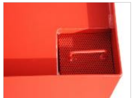
Suction opening and level indicator
