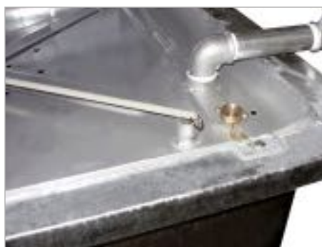
Dipstick to control the fill level
