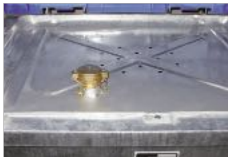
Fill tray and 2" tank truck coupling
