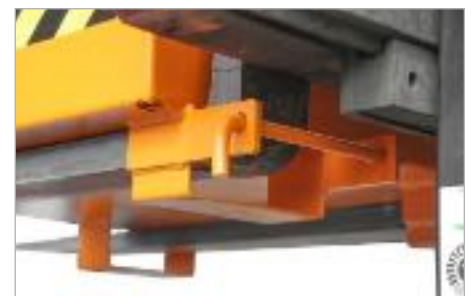
Secured by bolt to prevent slipping
