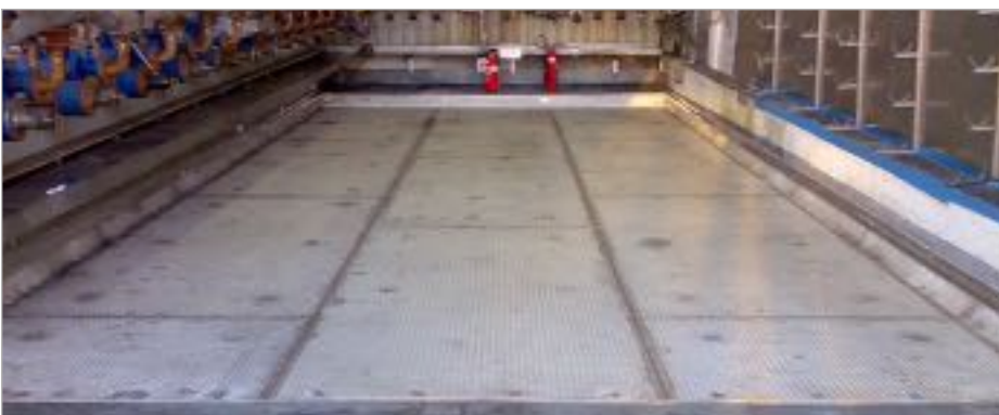
Ground protection floor elements made of stainless steel
