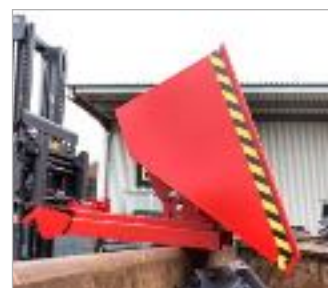
Emptied by activating release point 2
